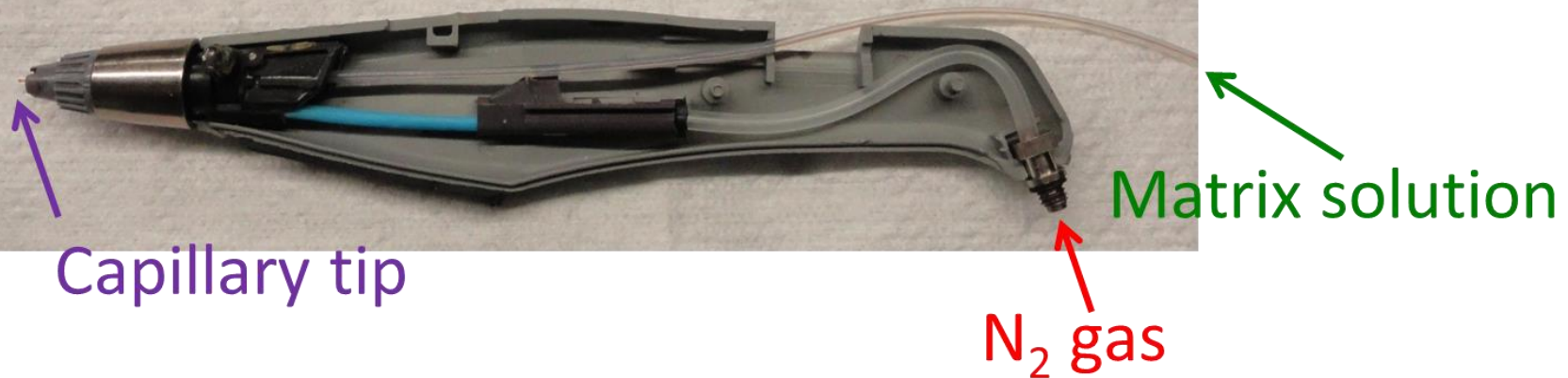
Fig. 4. Photograph showing modifications to an Aztek A470 airbrush (Testor, Rockford, IL) to create an oscillating capillary nebulizer. The trigger mechanism has been removed and a capillary has been run through the housing and out the spray tip. The capillary is run through plastic tubing (0.0625" o.d. x 0.02" i.d.) and nitrogen gas is supplied using the airbrush gas interface. Matrix solution is delivered through the capillary by means of a syringe pump.
